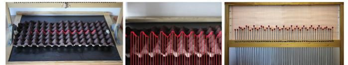
set-up with pinboard and laser line (left), laser line-based SR estimation (middle) and pinboard SR measurement (right).
